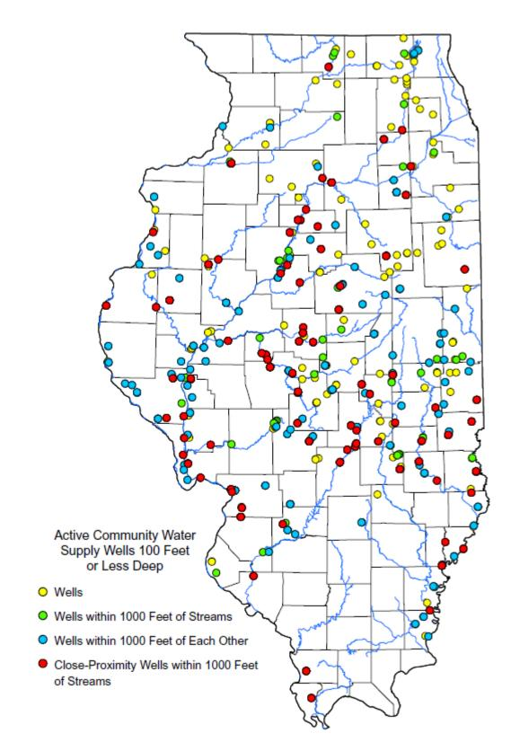
Figure 4. Community water supplies less than 100 feet deep, within 1000 feet of another community well, and within 1000 feet of a recognized stream (from Winstanley et al., 2006)
