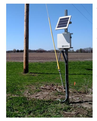
The rest of the monitoring wells were transducer stations that are more reliable for water level monitoring
